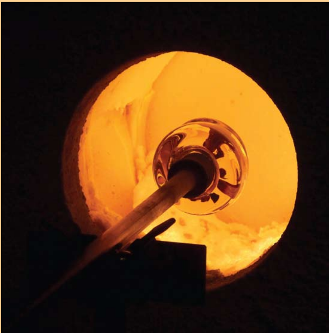
Once the design is picked up from the plate, the surface is fire polished in the glory hole.
