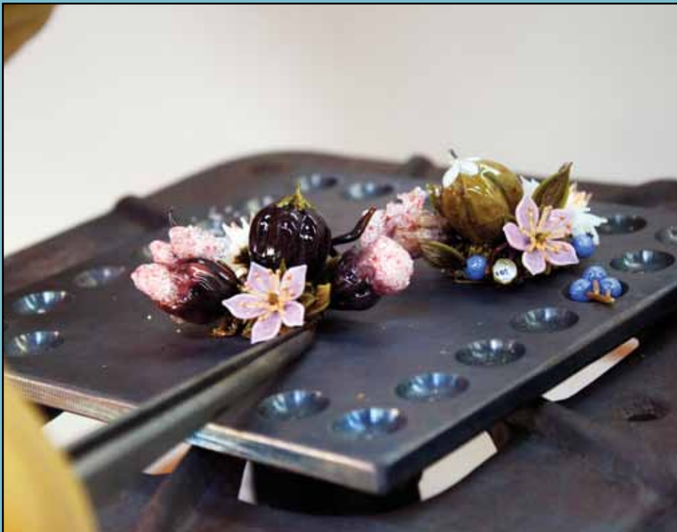
Preheating colored glass components on a gas fired hot plate. Photo by Lauren Ashley Garcia
