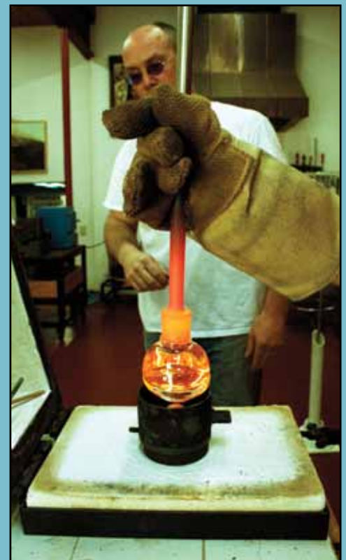
Dropping hot clear glass on colored glass in a suction cup. Photo by Lauren Ashley Garcia
